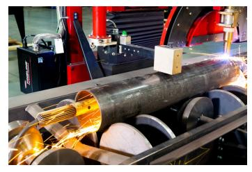
The high quality rotation joint with heat sink allows for cutting in high current applications without becoming dangerously hot to the operators touch.
